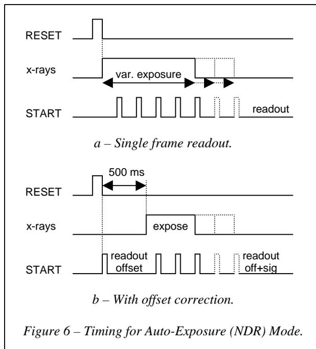
Figure 6 – Timing for Auto-Exposure (NDR) Mode.
