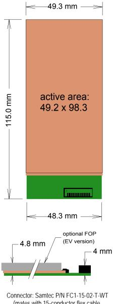
(mates with 15-conductor flex cable, Samtec P/N FJ-15-D-x.xx-4)
